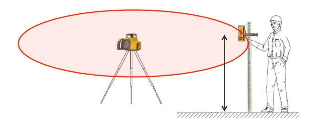
Laser receivers are used to level forms, concrete and dirt.
